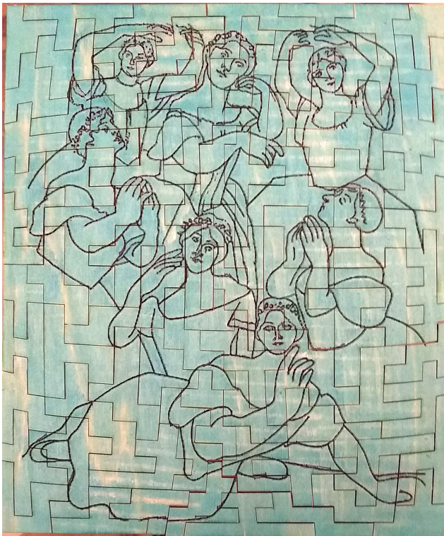
80-Piece puzzle with simpler part shapes, using a slight curve warping of the grid, 8×10 inches. (Etched image is Seven Ballerinas by Picasso.)
